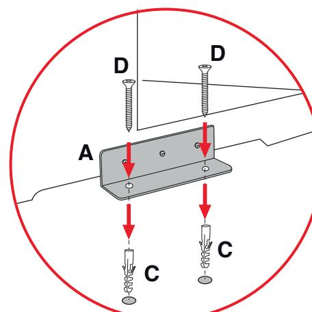
Insert the 2 screw anchors (C) in the holes made in the flooring and use a screwdriver or electric screwdriver to fix the plates with the 2 screws (D) supplied.
